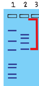
Figure 6: Measure distance migrated from the lower edge of the well to the lower edge of each band.
