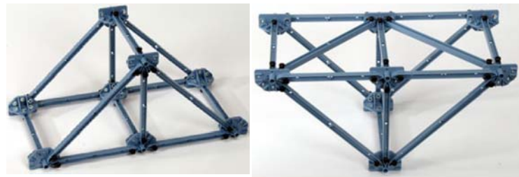
Figure 14: (Left) A three-dimensional kingpost truss structure. (Right) Kingpost truss with cross bracing.
