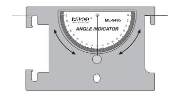
attached to a PASCO Dynamics Cart, by sliding the device into the slots on the top of the cart. It is necessary to adjust the thumbscrew and square nut as far up as possible on the Angle Indicator.
