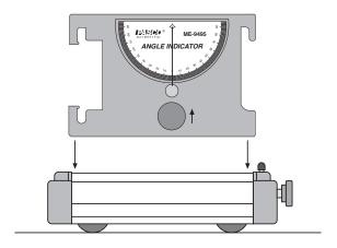
• attached to the side of a PASCO Dynamics Track.
