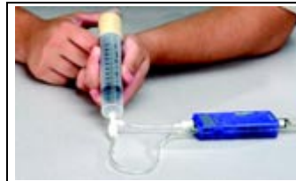
Figure 1: Measuring Pressure and Temperature Changes in the Ideal Gas Law Syringe
