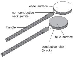
➤ NOTE: Oil build-up on the non-conductive neck can affect results. Clean with alcohol before using.
