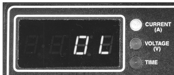
Display shows current Over Load
