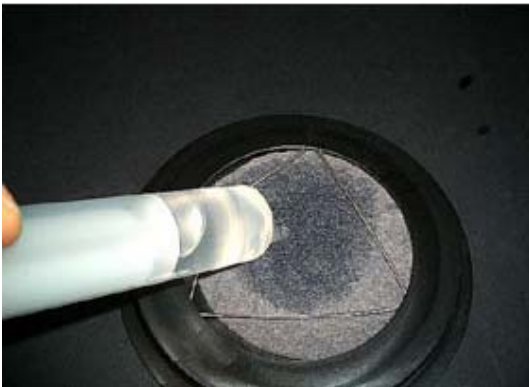
Fig. 2 Application of isopropanol or ethanol to the felt in the receptacle lid
