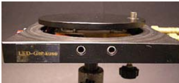
Fig. 6 Connections for plug-in LED illumination
